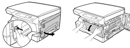
Gently pull the TD cartridge out while pressing the lock release button. Dispose of the old TD cartridge in accordance with local regulations.
